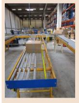
6. Package placed on a conveyor belt to check its weight, then taken to the palletisation station
